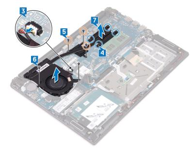
7 Lift the heat-sink assembly off the system board.
