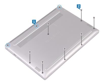
**3** Using your fingertips, pry the base cover off the palm rest and keyboard assembly.
