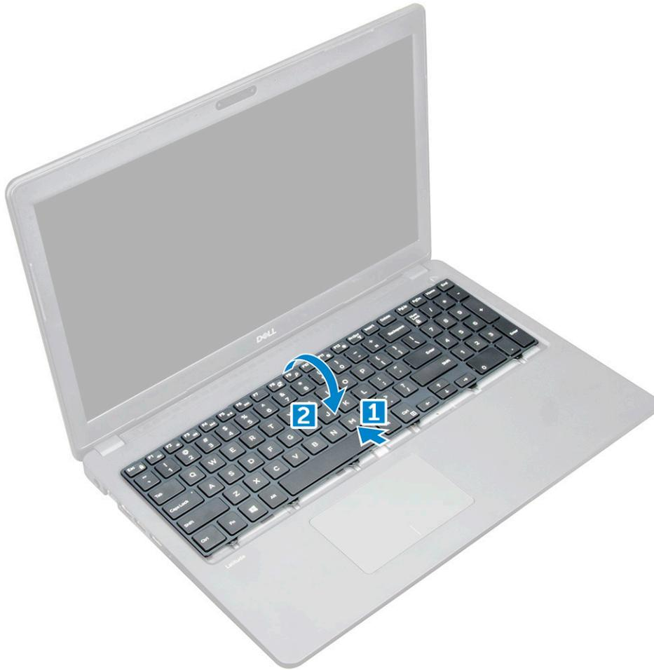
5 Then, disconnect the backlight connector [1] and the keyboard connector [2].
