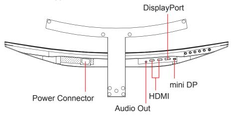
3.A. Please do not connect the DisplayPort out on the monitor to the DisplayPort or mini DP connector on the computer. DisplayPort out is used for daisy chain connection (Explained in section C)
