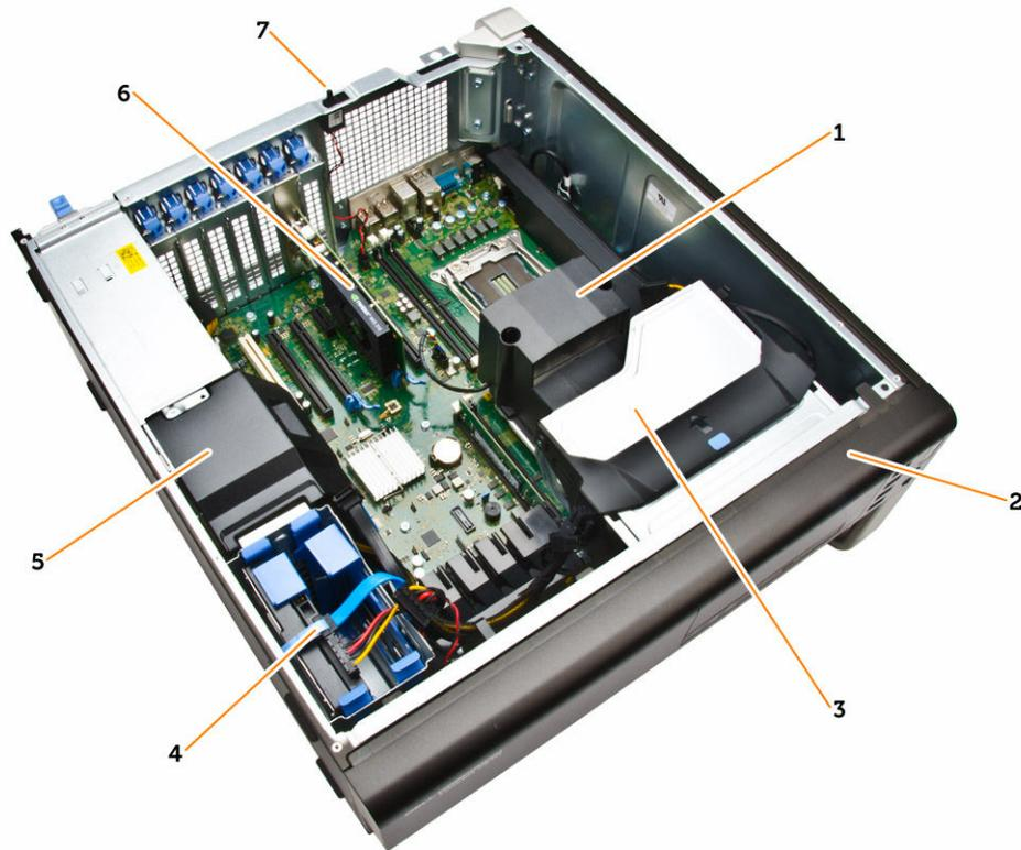
**Figure 2. Inside View of T7810 Computer**
