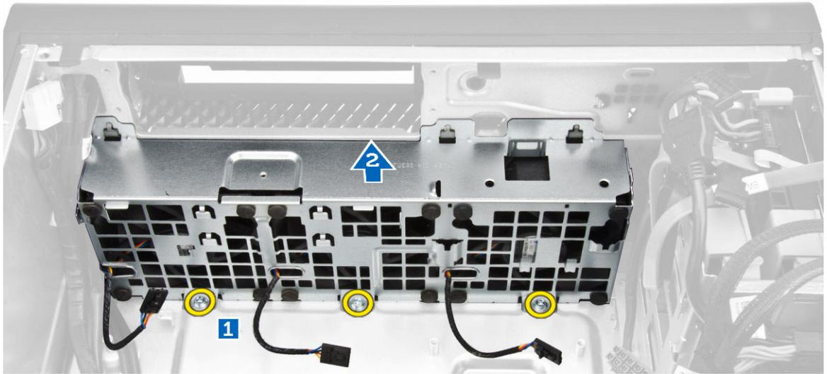
6. Pry away the grommets to remove the system fans from the system-fan assembly.
