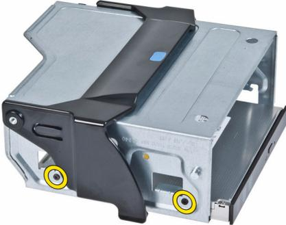
11. Remove the optical drive from the optical-drive cage.
