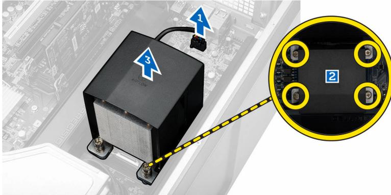
4. Repeat **Step 4** to remove the second heatsink module from the computer.
