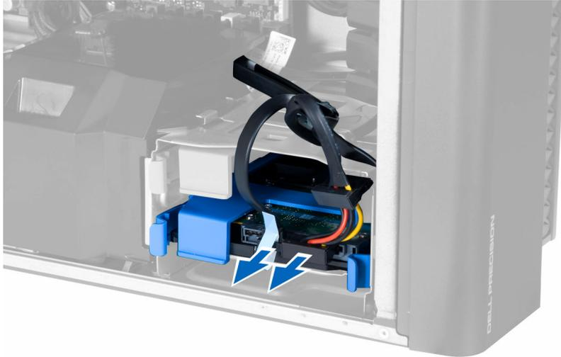
4. Press in on the latches on both sides of the hard-drive bracket.
