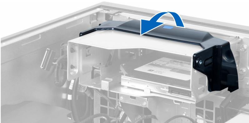
8. Holding the release latch, slide the optical-drive cage from the optical-drive compartment.
