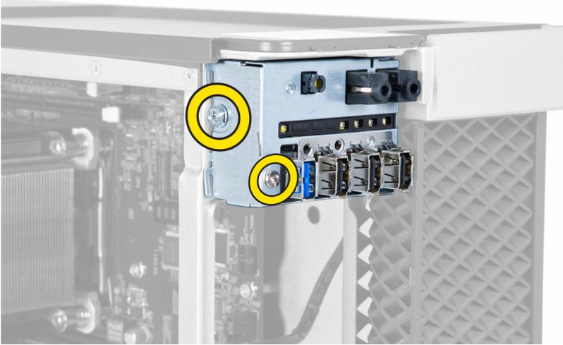
4. Remove the I/O panel cage from the chassis.
