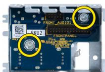
7. Remove the I/O panel from the I/O panel cage.
