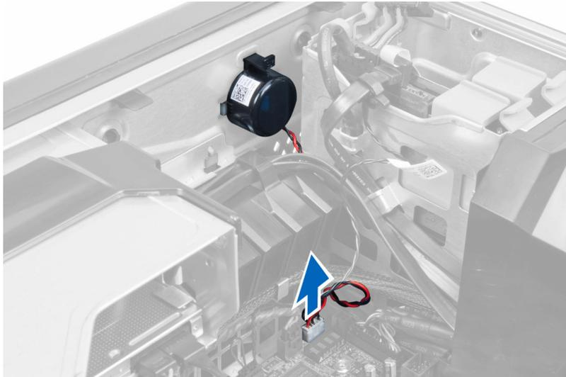
4. Press down the clasp, lift and remove the speaker.
