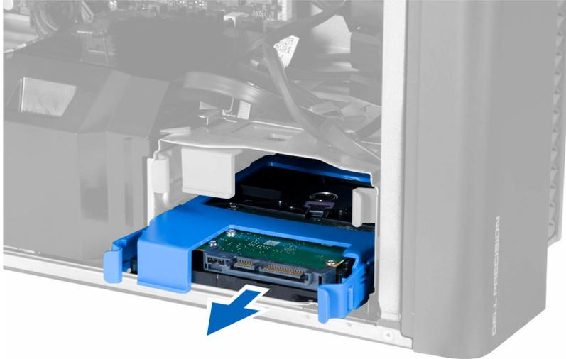
6. If a 2.5-inch hard drive is installed, remove the screws and lift up the drive to remove it from the hard-drive caddy.
