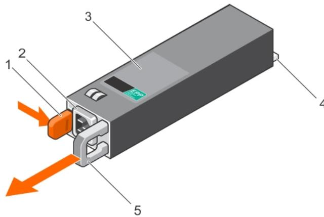
**Figure 33. Removing a redundant PSU**
