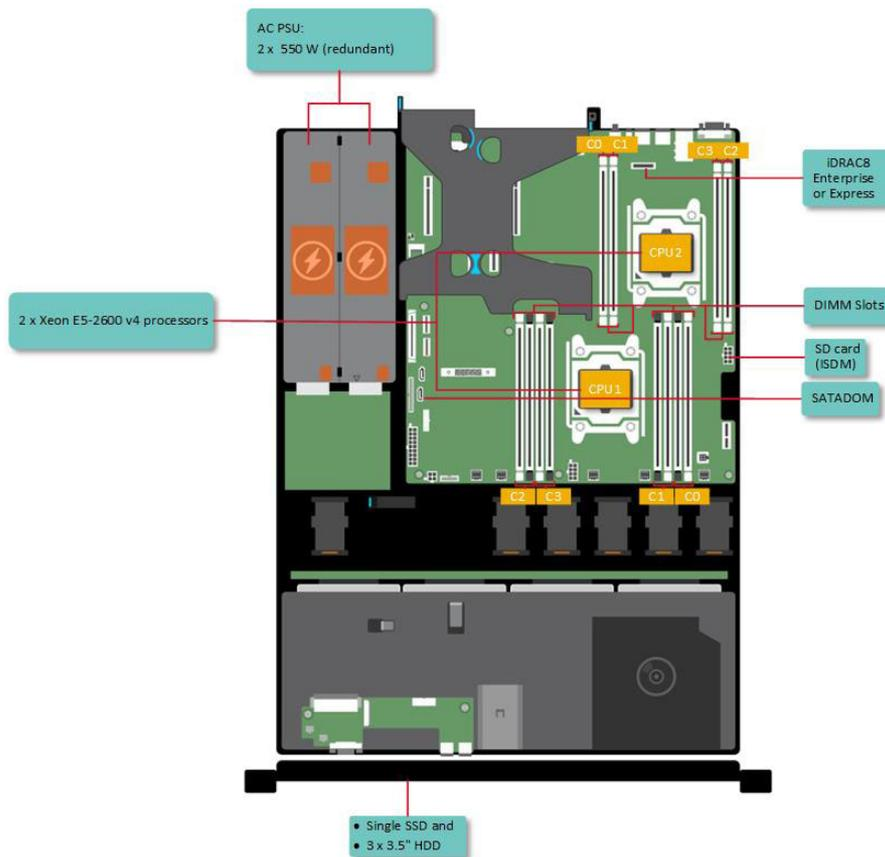
**Figure 1. Supported configurations for XC430 Xpress**
