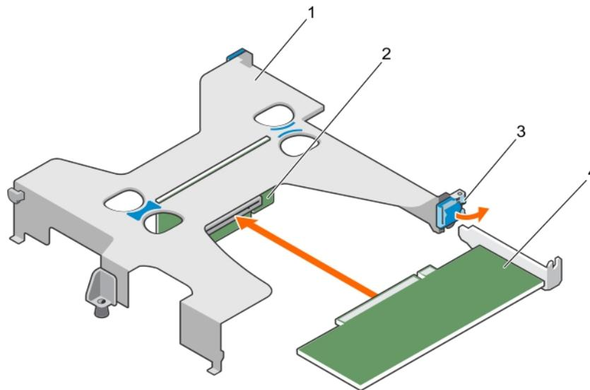
**Figure 30. Installing an expansion card into the expansion card riser**
