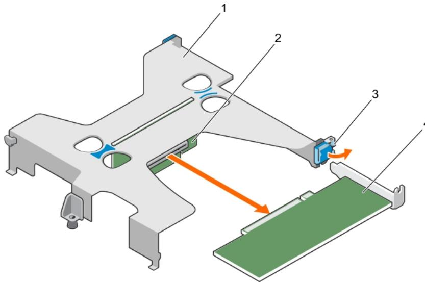
**Figure 29. Removing an expansion card from the expansion card riser**
