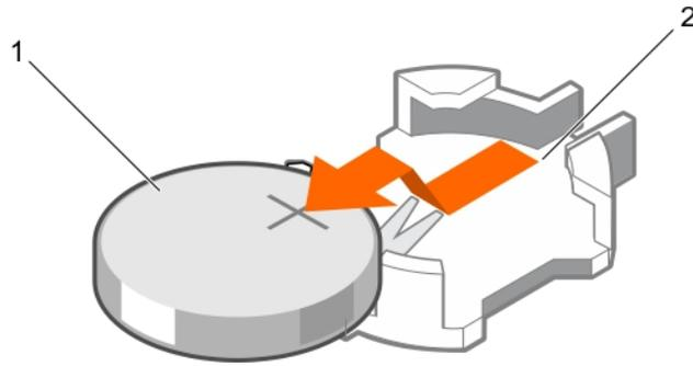
**Figure 35. Removing the system battery**
