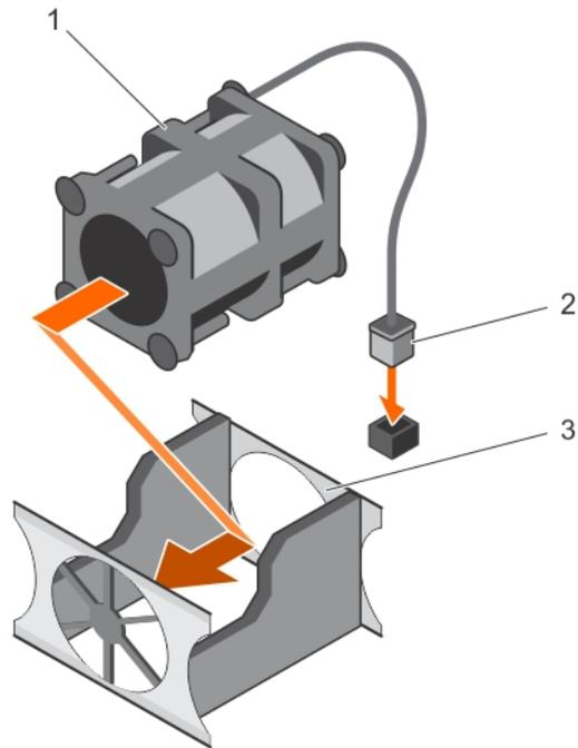
**Figure 25. Installing a cooling fan**
