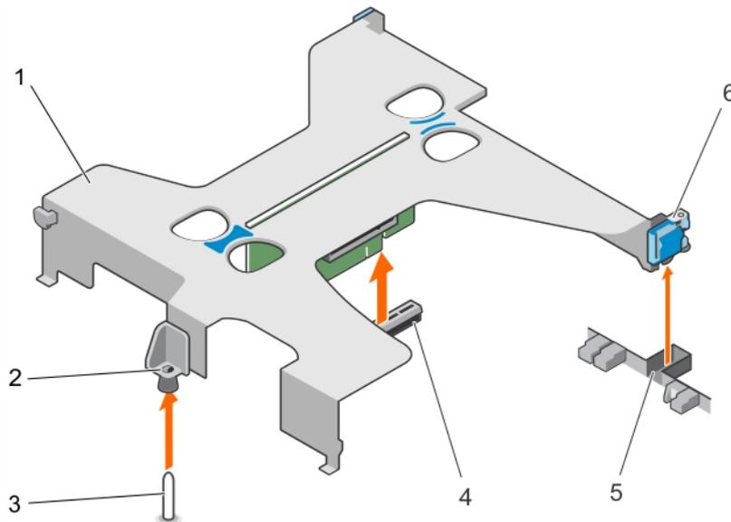
**Figure 27. Removing the expansion card riser**
