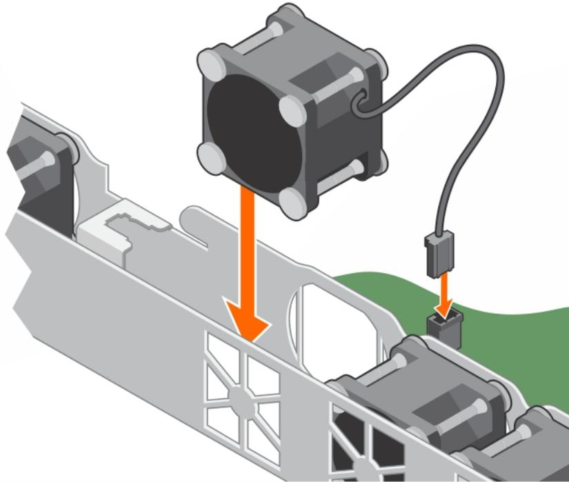
**Figure 26. Installing a cooling fan**
