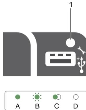
**Figure 7. iDRAC Direct LED indicator**
