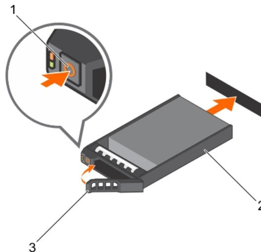
**Figure 21. Installing a hot swappable hard drive carrier**
