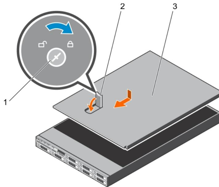
**Figure 12. Installing the system cover**
