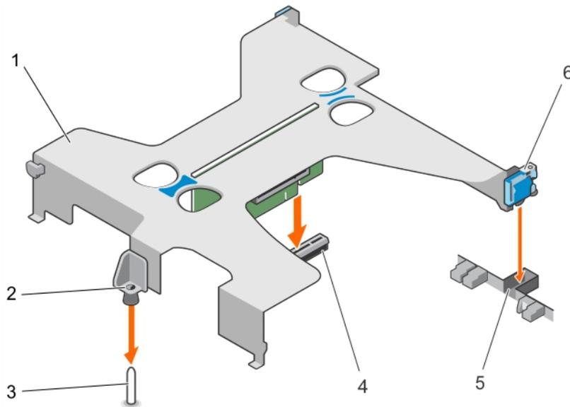
**Figure 28. Installing the expansion card riser**
