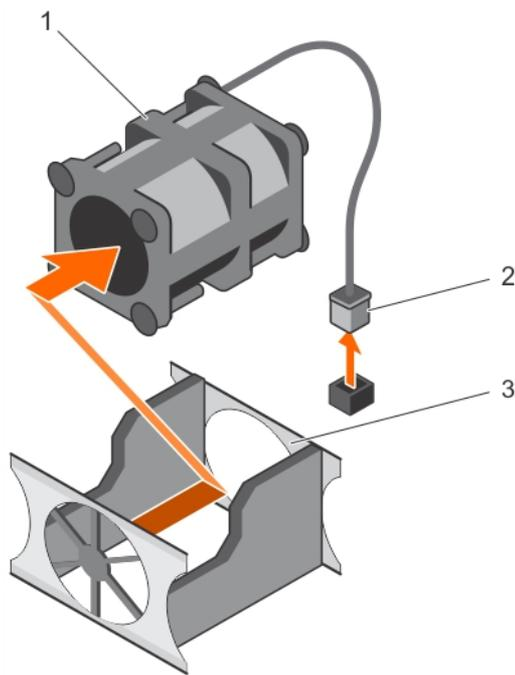
**Figure 24. Removing a cooling fan**
