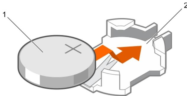
**Figure 36. Installing the system battery**
