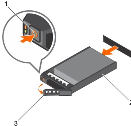
**Figure 20. Removing a hot swappable hard drive or SSD**
