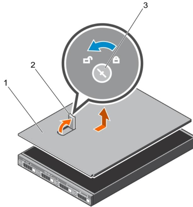
**Figure 11. Removing the system cover**
