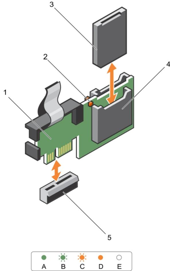
**Figure 31. Removing the internal SD module (ISDM)**
