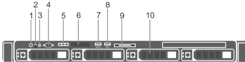
Figure 2. Front-panel features and indicators
