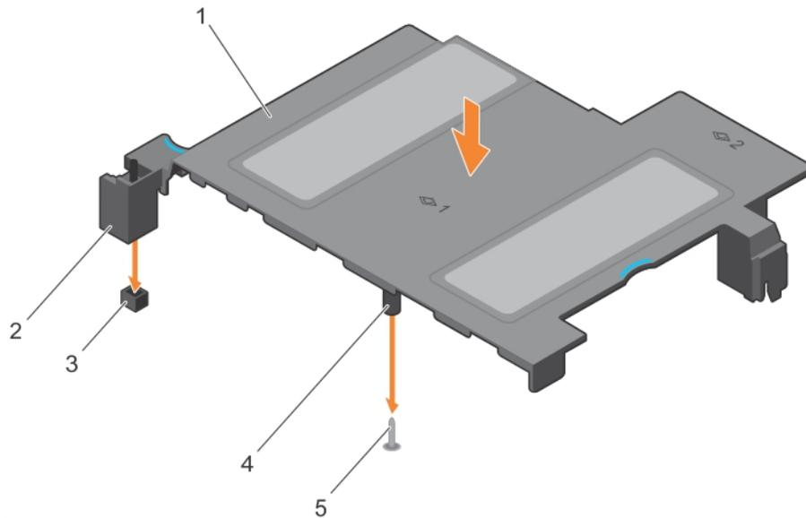
**Figure 15. Installing the cooling shroud**
