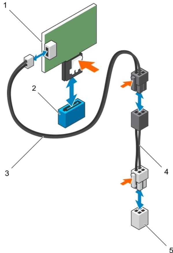
**Figure 19. Removing and installing SATADOM**
