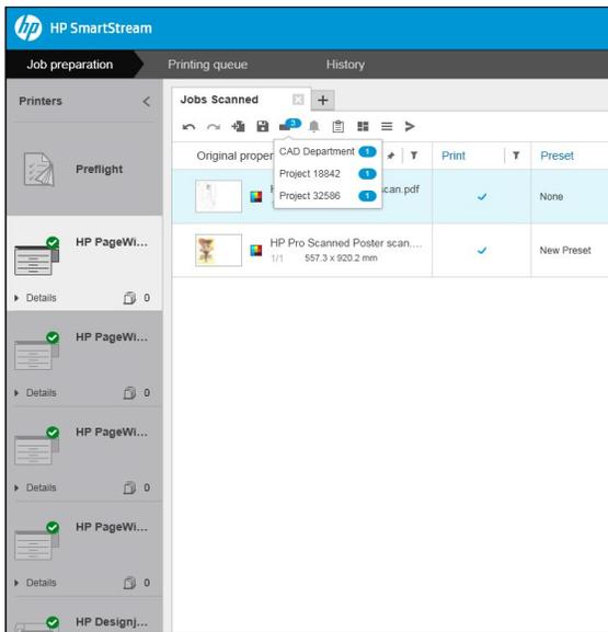
3. Act on a notification that a new job has arrived in a hot folder by adding it to the preparation pane. All settings defined in the Submission driver will be applied automatically.
