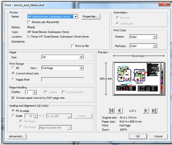
1. Send a file to print from any application and file format (.DWF file in the example), selecting HP SmartStream Submission driver from the printer dropdown menu.
