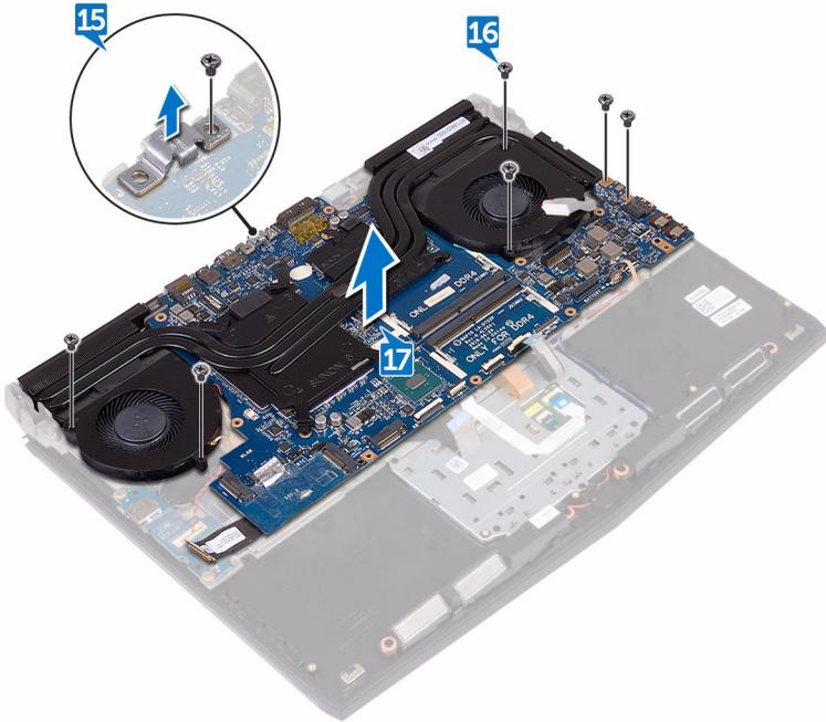
**18** Remove the [heat-sink assembly](#).
