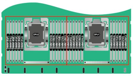
Figure 6-1 DIMM slots
