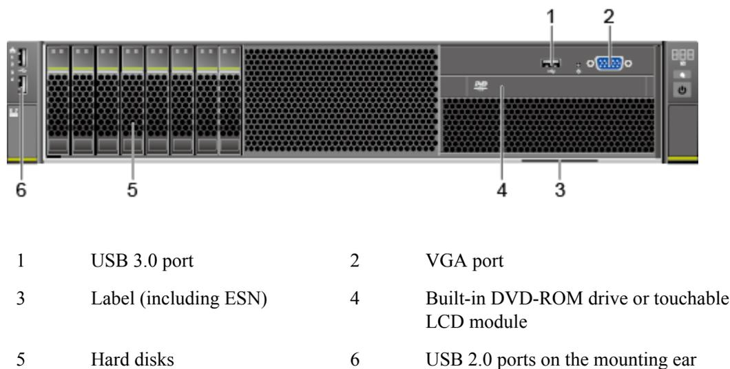
**Figure 4-2** shows the components on the front panel with 25 SAS/SATA hard disks.
