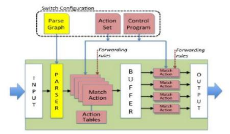
The switch needs to parse protocol packets. The protocol parser of traditional ASIC or OpenFlow1.x switches can only resolve known protocols. When the switch receives a packet of a new protocol, for example, an IPv8 packet, the protocol parser cannot parse the packet and discards the packet. OpenFlow2.0 defines a programmable protocol parser, which allows
