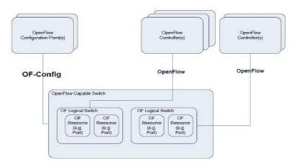
As shown in the figure, an OpenFlow-capable switch can be virtualized into multiple OpenFlow logical switches. To enable the logical switches and controllers to work properly, the OpenFlow Configuration Points module must perform the following configurations on the switches through the OF-Config protocol:
