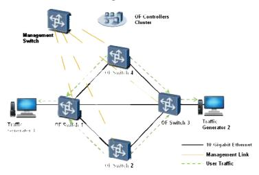
As shown in the figure, all switches communicate with the OpenFlow controller through a management switch. Four OpenFlow switches constitute a ring network through which two traffic generators send data to each other. The controller displays the global network topology. When a link is overloaded, the OpenFlow controller switches traffic to a lightly loaded link.
