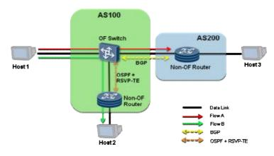
The complete transition from traditional networks to SDNs requires a fairly long period of time, so the SDN and traditional IP networks must be interoperable. In the figure, an OpenFlow switch communicates with two non-OpenFlow routers through BGP, OSPF, and RSVP-TE. All protocol packets are processed by the controller.
