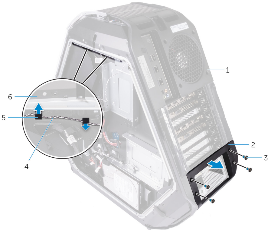
Figure 68. Removing the rear I/O accessibility lighting cable
