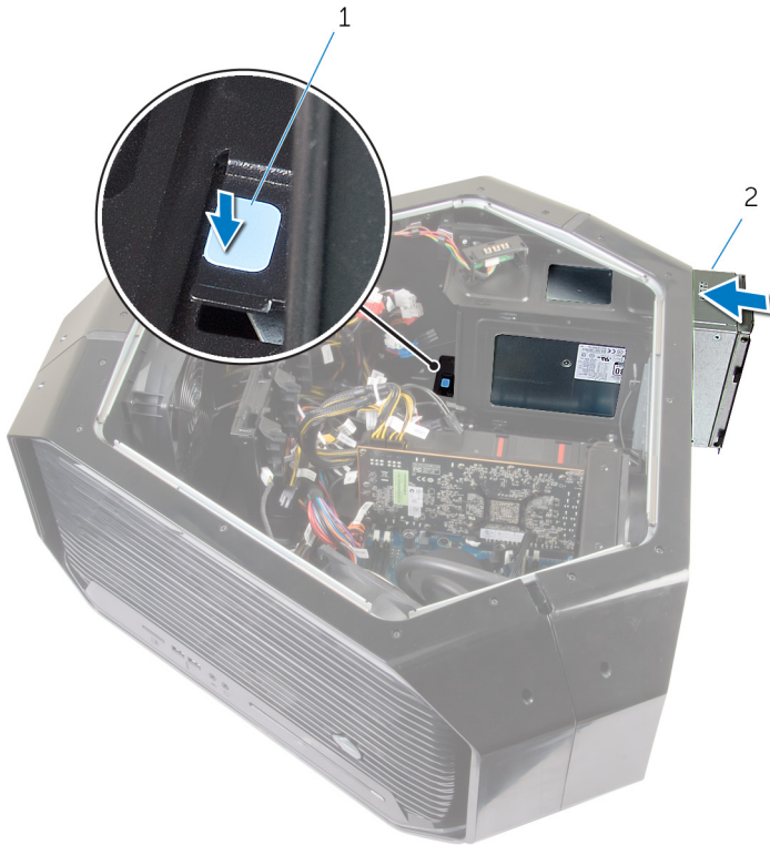
Figure 52. Replacing the power-supply unit
