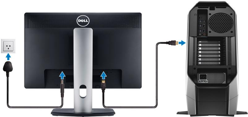
**NOTE:** The DisplayPort on the back panel of your computer is covered. Connect the display to the discrete graphics card of your computer.
