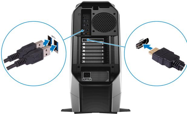
**NOTE:** Connect the headset to the HDMI port on the discrete graphics card and connect the display to any available port on the card.
