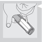
9 Pry the 2 AA-sized cylindrical nickel metalhydride batteries loose by inserting the screwdriver on the sides of the two batteries in the locations shown in the figure.
