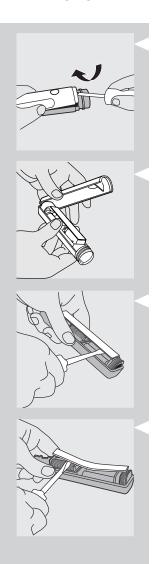
5 Now use the screwdriver as a lever to pry the 2 handle sections apart.
