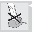
When the handle is placed incorrectly in the charger, the charge indicator light may still illuminate, but charging will not take place.
