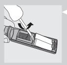
10 Use a twisting and prying motion to break the glue bond around the batteries. The 2 batteries are joined together with glue and will be lifted out together.
