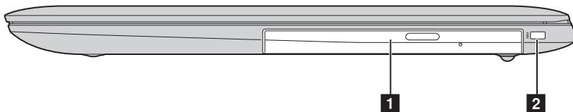
**1 Optical disc drive** Reads/Burns optical discs.
