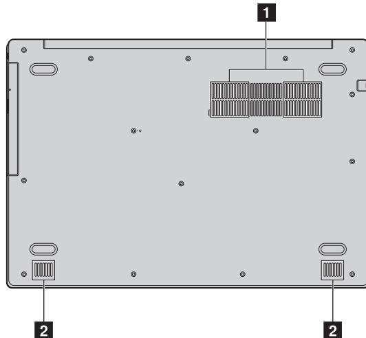
**1 Ventilation slots** Dissipate internal heat.
