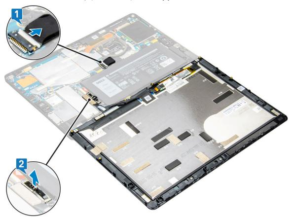
9 Lift the display assembly from the tablet.
