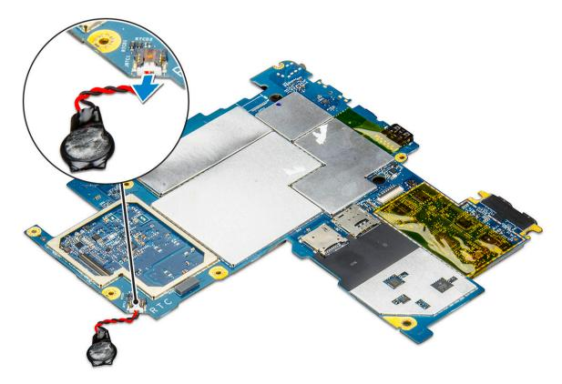
NOTE: If you can easily disconnect the RTC battery cable from beneath the connector on the system board, you need not remove the system board to remove the RTC battery.
