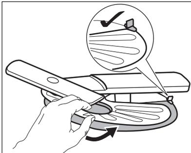
7. Reassemble the filters (B) and (C).
