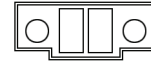
Fig. 16. Terminal block for connection to the inverter shut-down auxiliary contact of the manual bypass board.
