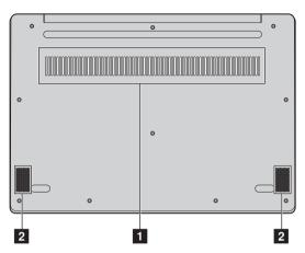
**1 Ventilation slots** Dissipate internal heat.
