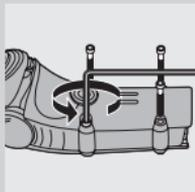
**2** Let the shaver run until it stops, undo the two screws in the hair chamber by means of a screwdriver and remove it.
