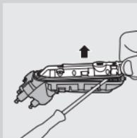
**7** Remove the back panel of the sealed power unit by means of a screwdriver.
