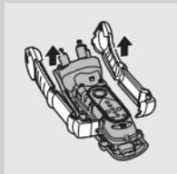
**3** Undo the four screws at the front of the shaver by means of a hexagon key and remove the front panel of the housing.
