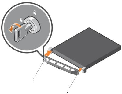
Figure 12. Installing the optional front bezel
