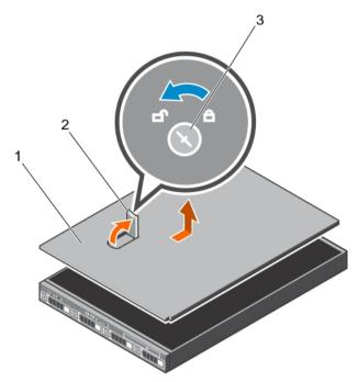
Figure 14. Removing the system cover
