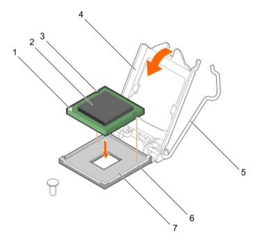
Figure 66. Installing a processor
