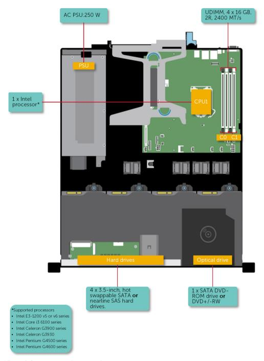
Figure 1. System view with supported configurations
