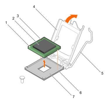
Figure 64. Removing and installing a processor
