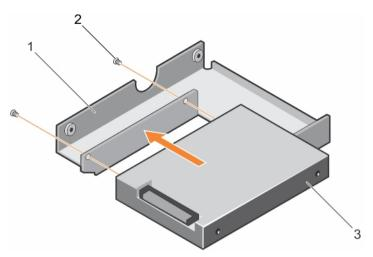
Figure 36. Installing a 2.5-inch hot swappable hard drive into a 3.5-inch hard drive adapter
