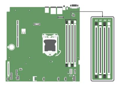
Figure 23. Memory socket locations on the system board
