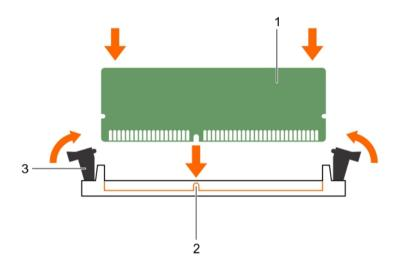
Figure 25. Installing the memory module
