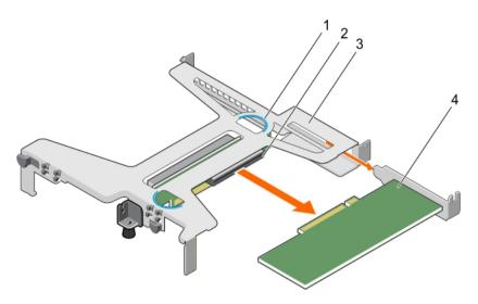
Figure 54. Removing the expansion card from the expansion card riser
