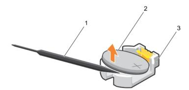
Figure 70. Removing the system battery
