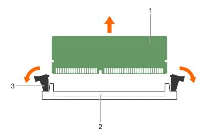
Figure 24. Removing the memory module
