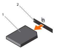
Figure 58. Removing the optional SD vFlash card
