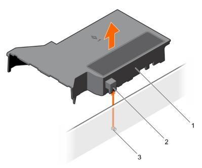
Figure 21. Removing the cooling shroud
