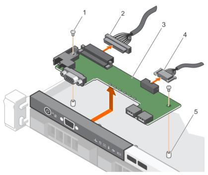
Figure 80. Removing the LED control panel board—four cabled hard drive chassis
