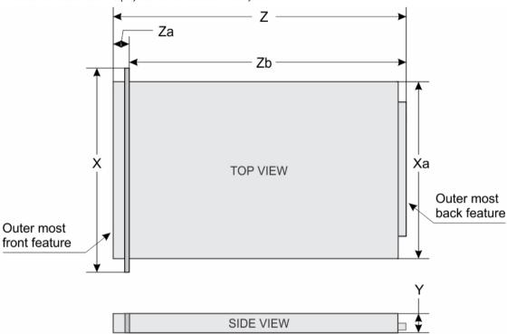
Figure 11. Chassis dimensions of the PowerEdge R230 system
