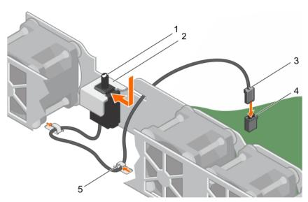
Figure 20. Installing the intrusion switch
