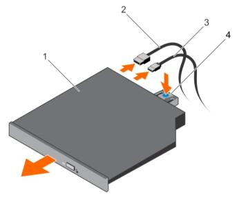
Figure 44. Removing the optical drive
