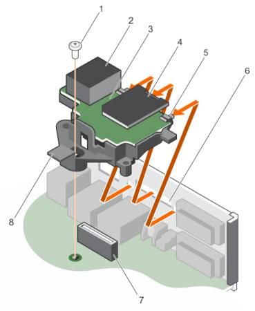
Figure 60. Removing the iDRAC port card
