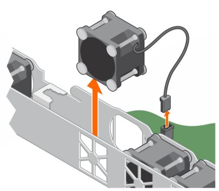
Figure 48. Removing a cooling fan
