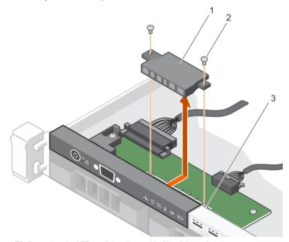
Figure 79. Removing the LED module—four cabled hard drive chassis
