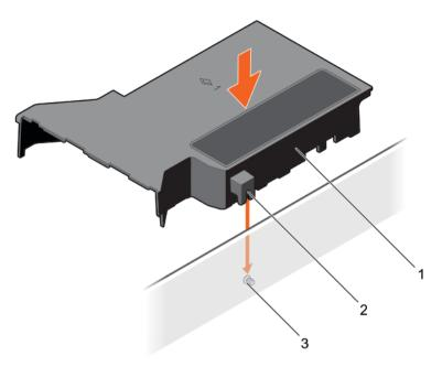
Figure 22. Installing the cooling shroud
