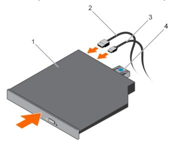
Figure 45. Installing the optical drive
