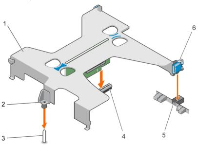
Figure 53. Installing the expansion card riser
