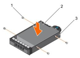
Figure 30. Installing a cabled hard drive to a cabled hard drive carrier
