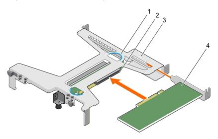
Figure 56. Installing the expansion card in the expansion card riser
