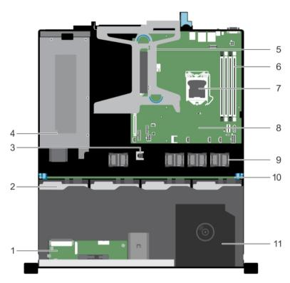
Figure 16. Inside the system—four 3.5-inch or 2.5-inch hot-swappable hard drive systems
