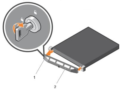
Figure 13. Removing the optional front bezel
