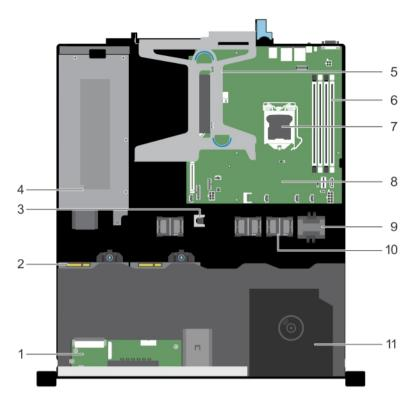
Figure 18. Inside the system—two 3.5-inch cabled hard drive systems
