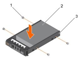
Figure 34. Installing a hot swappable hard drive into a hot swappable hard drive carrier
