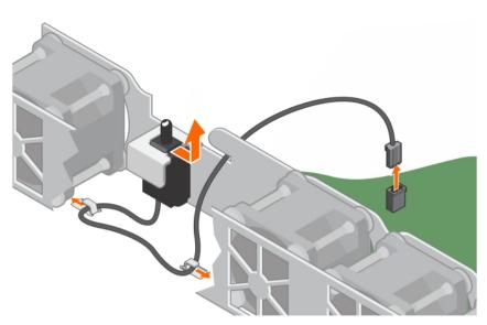
Figure 19. Removing the intrusion switch
