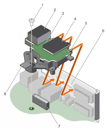
Figure 61. Installing the iDRAC port card
