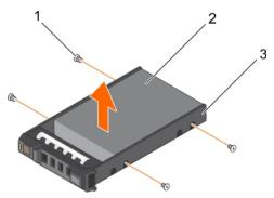
Figure 33. Removing a hot swappable hard drive from a hard drive carrier
