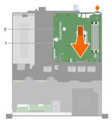
Figure 84. Removing the system board
