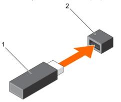
Figure 51. Installing the internal USB memory key
