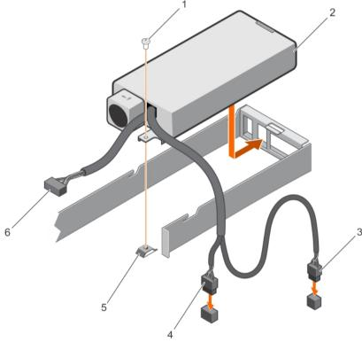
Figure 69. Installing a cabled PSU
