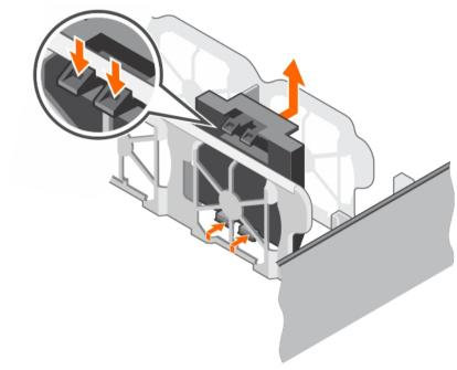
Figure 46. Removing a cooling fan blank
