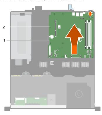
Figure 85. Install the system board
