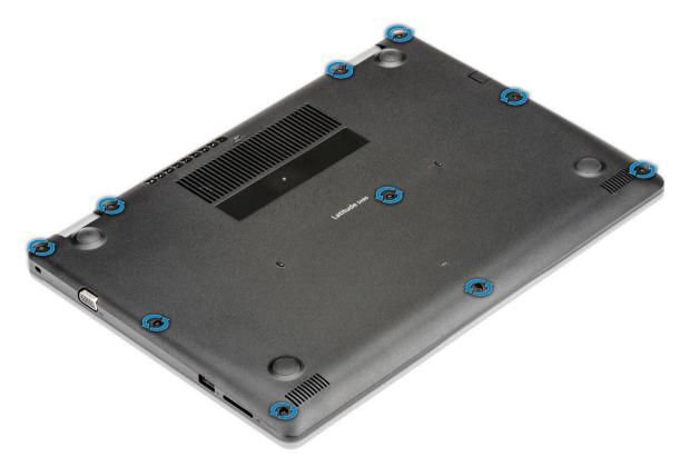
b Pry the base cover from the upper right edge [1] and continue to pry the outer edges of the base cover in clockwise direction [2].
