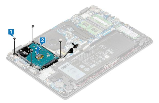
4 Disconnect the HDD cable interposer.
