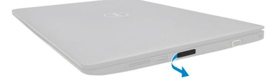
3 Insert the tip of a paperclip into the hole of the SIM tray slot and then pull out and remove the SIM tray.
