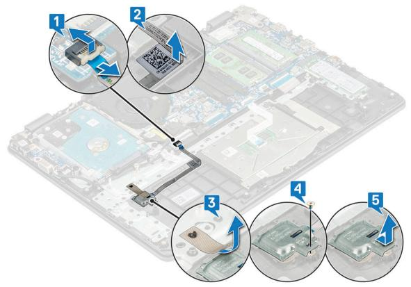
d Lift the fingerprint reader off the computer
