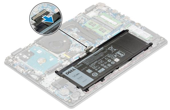
b Remove the 5 M2x3 screws that secure the battery to the computer [1].
