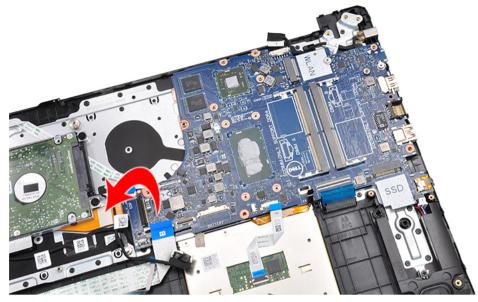
2 Disconnect the WWAN daughter board FPC [1] and VGA daughter board cable [2] from the connectors on the bottom side of
