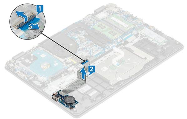
b Remove the two M2x3 screws that secure the I/O board to the system [1] and lift the I/O board off the palmrest [2].
