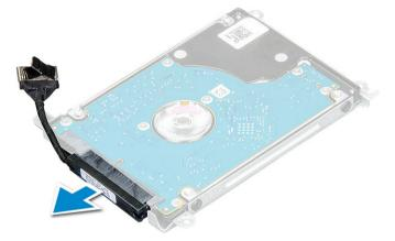
5 Then, remove the M3x3 screws to detach the bracket from the HDD.
