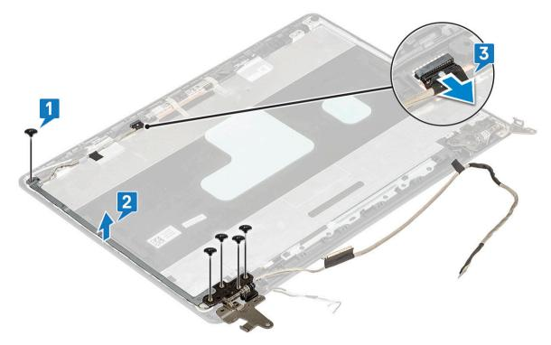
5 Peel the adhesive tapes securing the display cable to the LCD back cover and unroute it from the routing channel.
