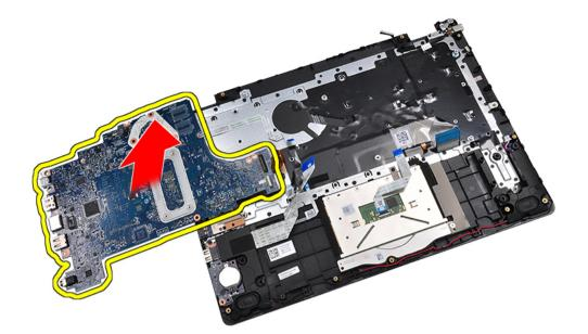
• For other configurations, lift the system board.
