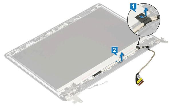
5 Then, remove the 4 M2x2 screws [1] securing the LCD panel to the LCD back cover and flip it over to expose the eDP cable connector [2].
