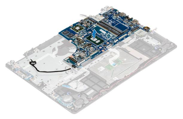
7 Remove the screw securing the USB Type-C bracket to the system board [1] and lift the USB Type-C bracket from the system board [2].
