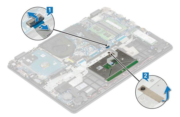
8 Remove the four M2x2 screws that secure the touchpad on the computer [1] and lift the touchpad from the system [2].
