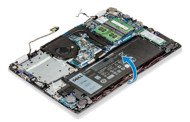
7 Remove the 5 M2.5x5 screws that secure the hinge brackets to palm rest [1] and lift the display assembly away from the computer [2].
