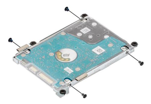
6 Lift the bracket from the hard drive.
