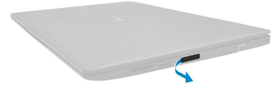
3 Insert the tip of a paperclip into the hole of the SIM tray slot and then pull out and remove the SIM tray.
