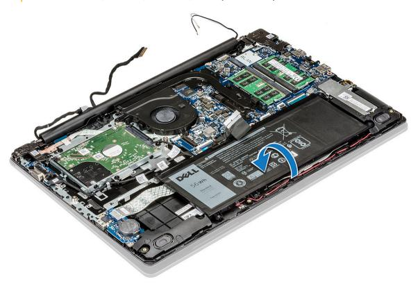
Remove the 6 M2.5x2.5 screws [1] and lift the display assembly away from the computer [2].
