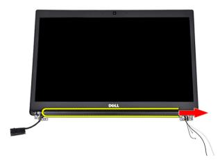
4 Remove the display hinge cap.
