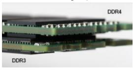
Figure 2. Thickness difference
