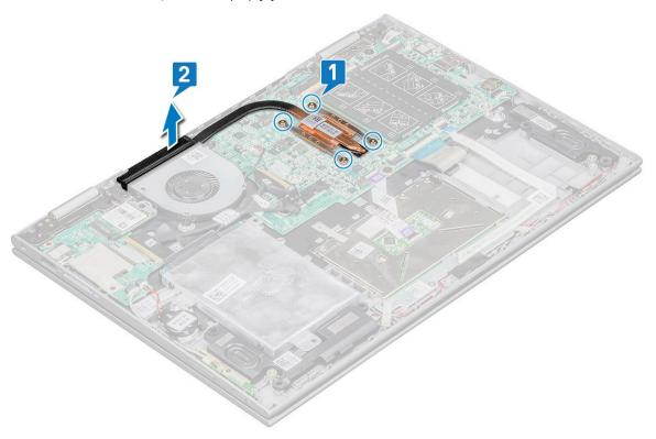
(i) NOTE: Ensure to loosen the screws diagonally. The screws cannot be removed completely as being retention screws.
