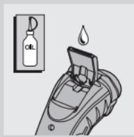
**3** Lubricate the trimmer teeth with a drop of sewing machine oil every six months.
