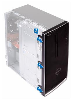
**2** Rotate and pull the front bezel away from the front of the computer to release the front bezel tabs from the front panel slots.
