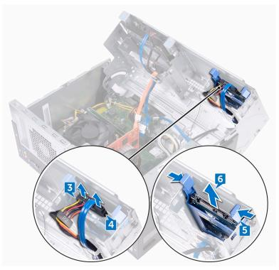
7 Pry the hard-drive bracket to release the tabs on the bracket from the slots on the hard drive.
