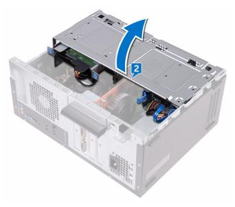
**3** Lift the tab to open the card-retention bracket.
