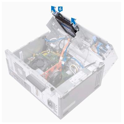
7 Remove the four screws (#6-32xL3.6) that secure the hard-drive bracket to the hard drive.
