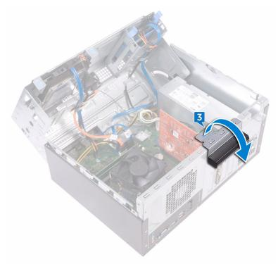
**4** Push the securing tab on the PCIe slot away from the graphics card.
