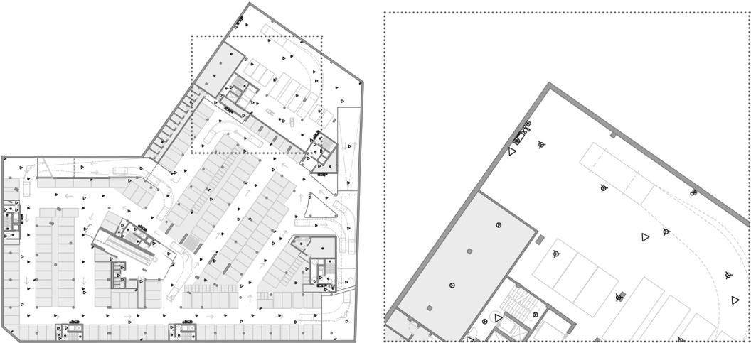
The diagram shows a floor plan of a building with a fire alarm system. On the left is a full view of the plan with a dashed black box highlighting a specific area. On the right is a magnified view of that area. In this magnified view, fire extinguishers are represented by black icons, and emergency lights are represented by black triangles. The extinguishers are placed at various points along the evacuation routes.
