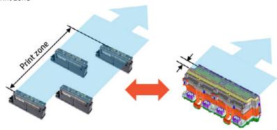
When the 4.25-inch printheads are configured to print two colors of ink, two printheads are required along the paper feed direction in a 4-color printing system. In HP's Color Inkjet Web Presses, this is implemented with two tandem printbars. Unlike HP 841 PageWide XL Printheads, HP's 4.25-inch printheads were not designed to directly stack together and so they must be staggered and offset as shown in Figure 4.
