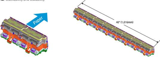
Two schemes for 4-color printing are shown schematically in Figure 4. Four HP 4.25-inch printheads produce an 8-inch print swath and two HP 841 PageWide XL Printheads produce a 10-inch swath. The arrangement of printheads is shown to relative scale.
