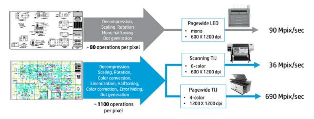
The modular architecture of the image processing pipeline for HP Pagewide XL Printers is shown schematically in Figure 8. Wider (or narrower) printbars can be built by adding (or removing) print module controllers. As with the printhead and ink supply modules, the image processing pipeline is modular and scalable along the printbar. By adding hub controllers for each printbar, multiple printbars can be supported in future product platforms.
