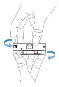
2. With the USB-C cable facing you, turn the top section to release the USB-C cable.
