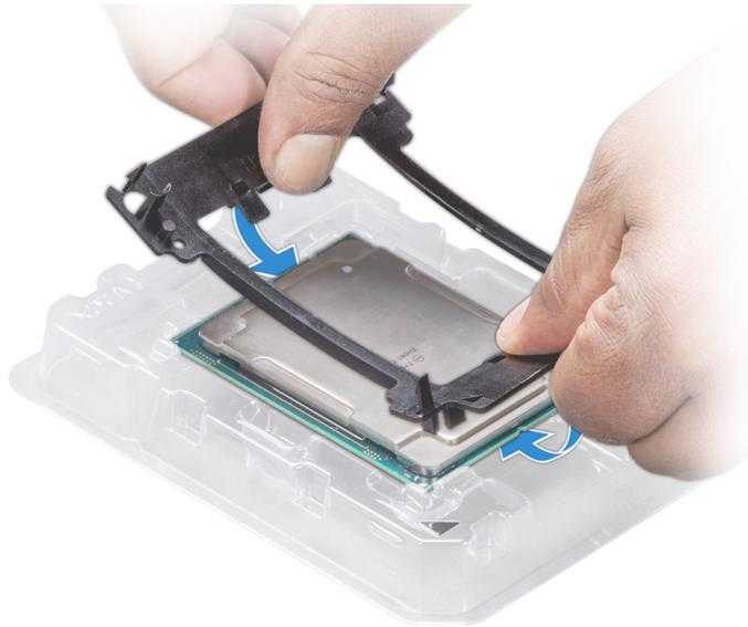
**Figure 14. Installing the processor bracket**
