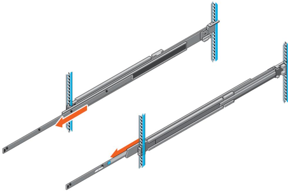
**Figure 25. Pull out inner rail**
