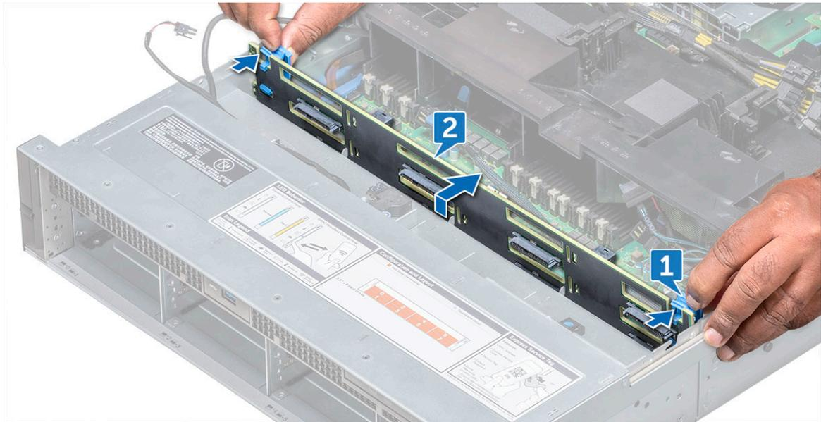
Figure 23. Removing hard drive backplane
