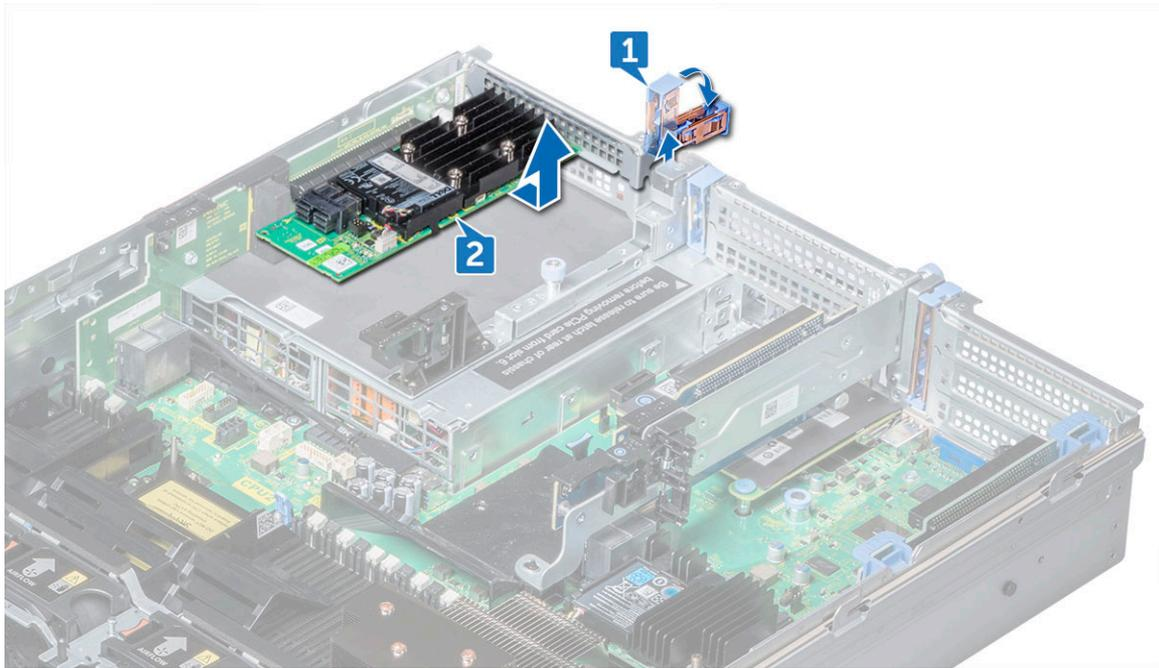
**Figure 19. Removing expansion card from expansion card riser 3**
