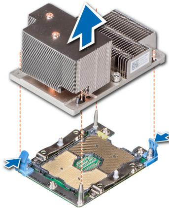
Figure 13. Removing heat sink (2U)
