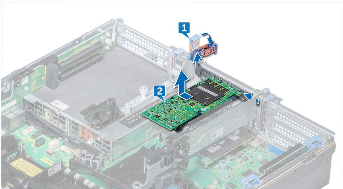
Figure 18. Removing expansion card from expansion card riser 2
