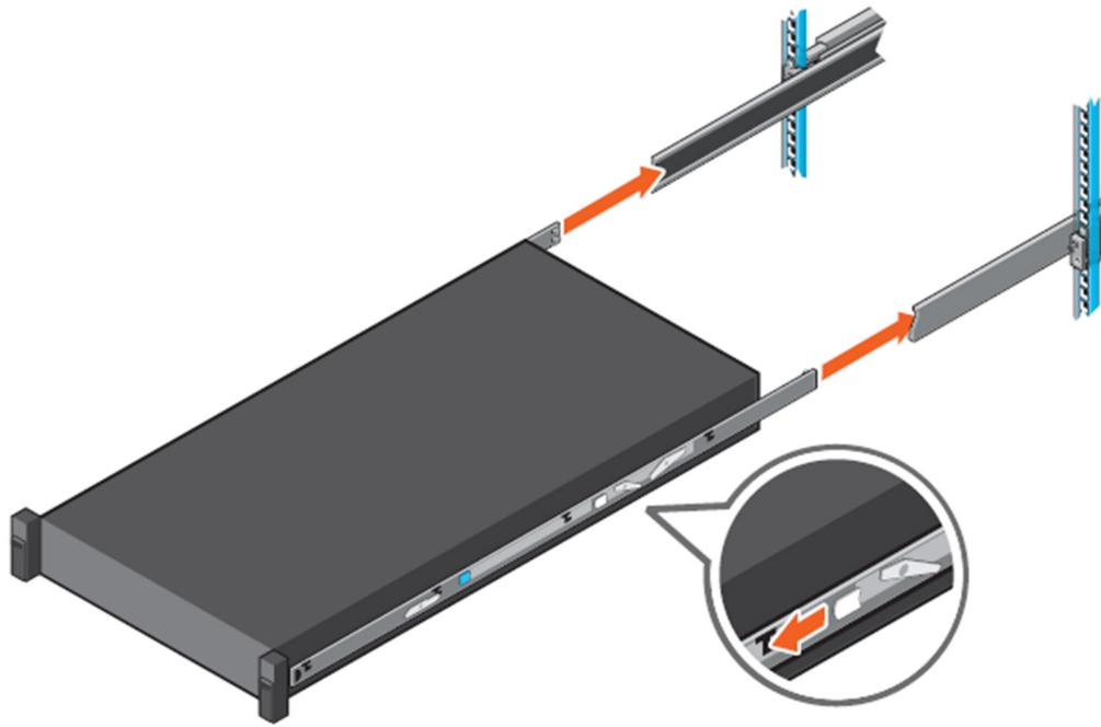
**Figure 30. Install system into the extended rails**
