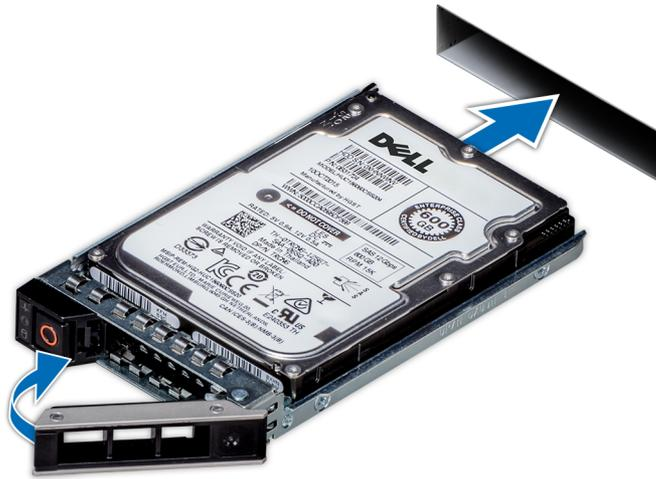
**Figure 11. Installing hard drive**
