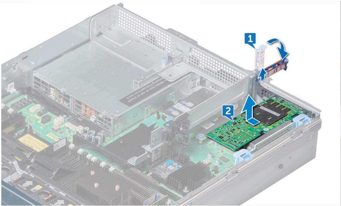
Figure 17. Removing expansion card from expansion card riser 1
