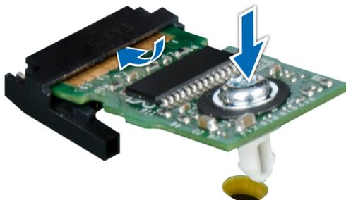
**Figure 33. Trusted platform module**
