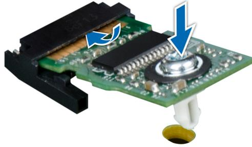
Figure 24. Installing the TPM
