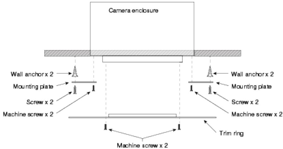
1. Attach the mounting plates to the camera with the black machine screws.
