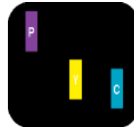
Two adjacent lit sub pixels: - Red + Blue = Purple - Red + Green = Yellow - + Blue = Cyan (Light Blue)
