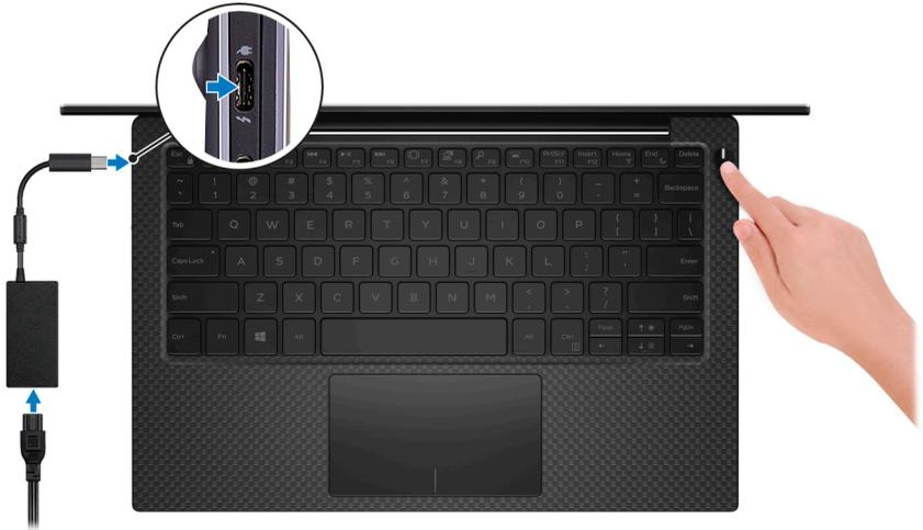
**NOTE:** To conserve battery power, the battery might enter power saving mode. Connect the power adapter and press the power button to turn on the computer.
