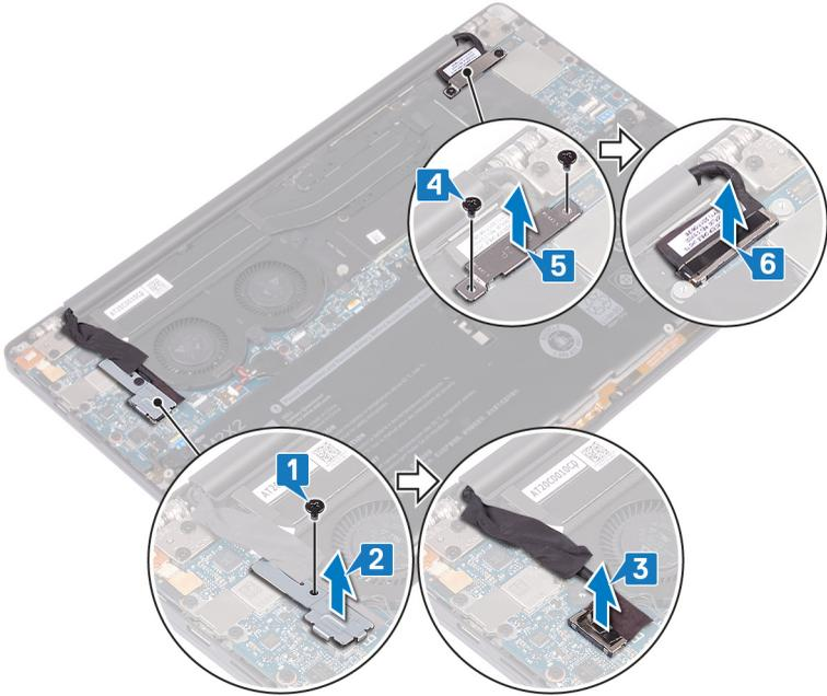
**7** Disconnect the antenna cables from the system board.
