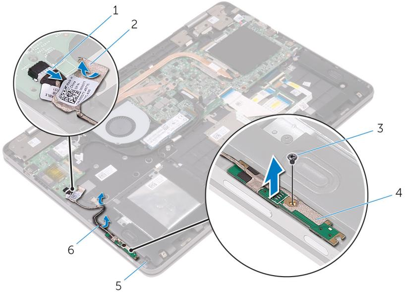
**Figure 22. Removing the power and volume-buttons board**
