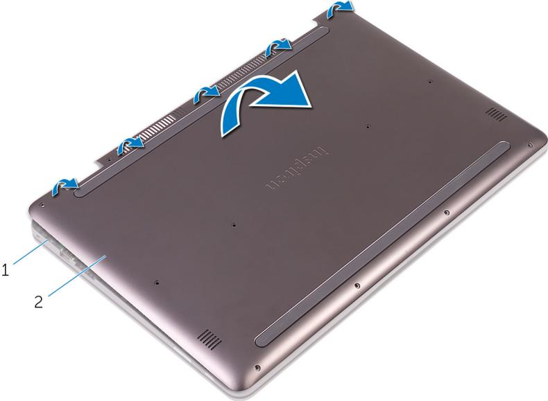
Figure 2. Removing the base cover
