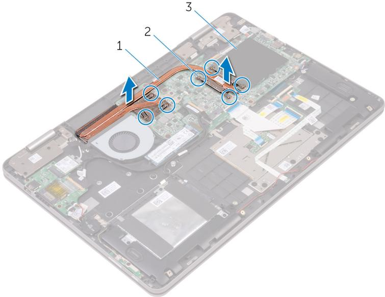
**Figure 20. Removing the heat sink**
