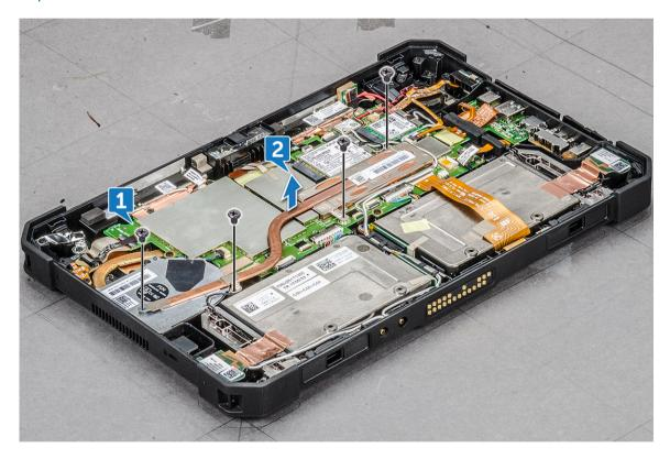
$\triangle$  CAUTION: When in use, the surface of the heat sink is hot. Ensure to lift the heat sink cautiously.
