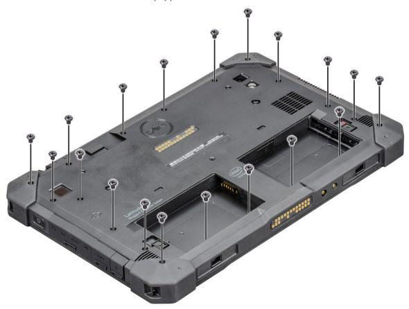
4 Flip the system so that the display assembly is at top view.
