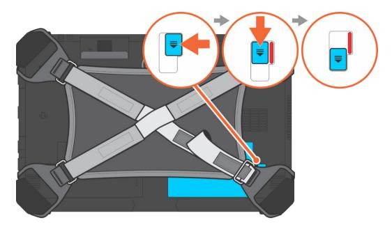
The battery is released from the battery bay.
