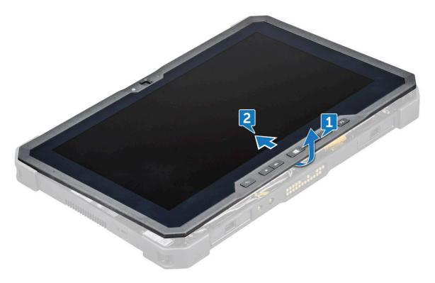
8 Flip the display assembly by an angle less than 90°.
