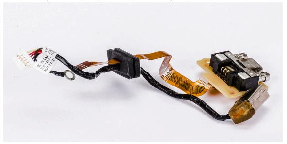
ONOTE: Malfunction of either component requires to remove both power connector port and micro serial port.
