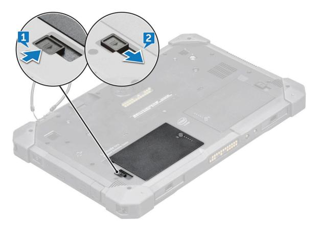
The battery is released from the battery bay.
