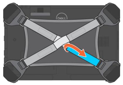
3 Slide the strap and release the strap from the holder to access the battery latch.
