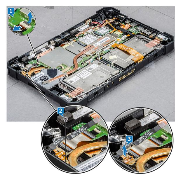
NOTE: NEVER pull the microphone by the cable. In case the circuit board is not released smoothly, push from below the microphone circuit board by a plastic scribe.
