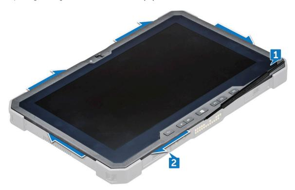
NOTE: Gently pry the edges evenly to unlock the plastic lock that secures the display assembly with the tablet chassis.
