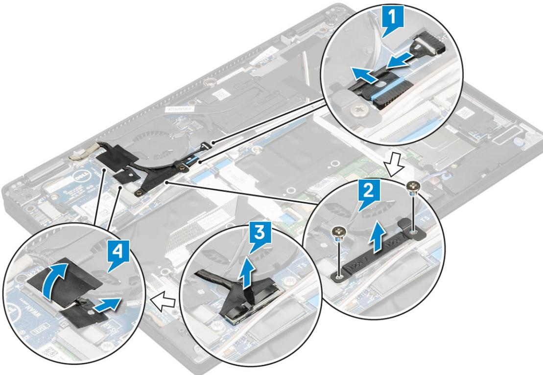
4 Disconnect the following cables from the system board .
