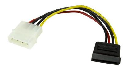
This 6in 4 Pin LP4to SATA power adapter cable features one 4 Pin LP4 male connector and one female SATA power connector, allowing you to power a Serial ATA hard drive from a conventional LP4 connection, eliminating the need to upgrade the computer power supply for compatibility with the SATA hard drive.
