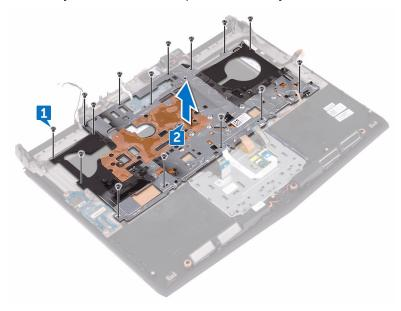
3 Lift the keyboard at an angle and remove it from the tabs on the palm-rest assembly.
