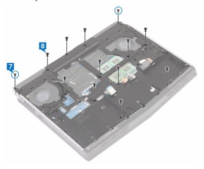
Lift the computer base off the palm-rest assembly.
