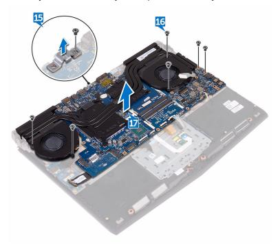
18 Remove the <u>heat-sink assembly</u>.
