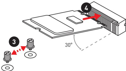
5. Put the screw in the notch on the trailing edge of your M.2 module and tighten it into the base screw.
