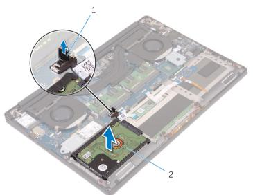
5 Disconnect the hard drive interposer from the hard drive assembly and then remove the hard drive covers away from the hard drive.
