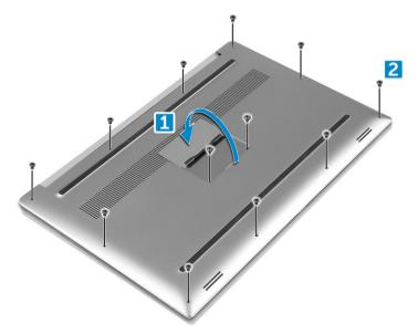
4 Pry the edges of the base cover and lift it to remove it from the computer.
