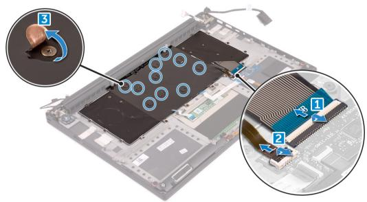
4 Un-route the LVDS cable [1] and then remove the 31 M1.6 x 1.5 screws that secure the keyboard to the computer [2].
