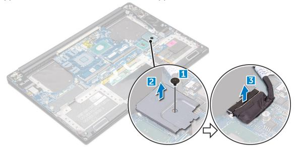
4 Slide out the connector latches to disconnect all the cables from the system board.
