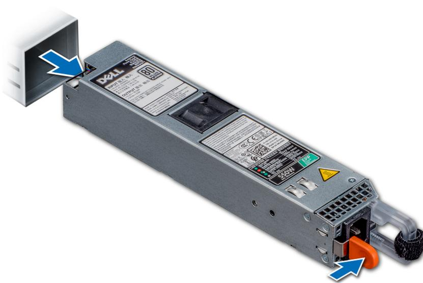
Figure 97. Removing a power supply unit
