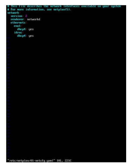
Figure 5. Configuring iDRAC interface to DHCP mode in Ubuntu
