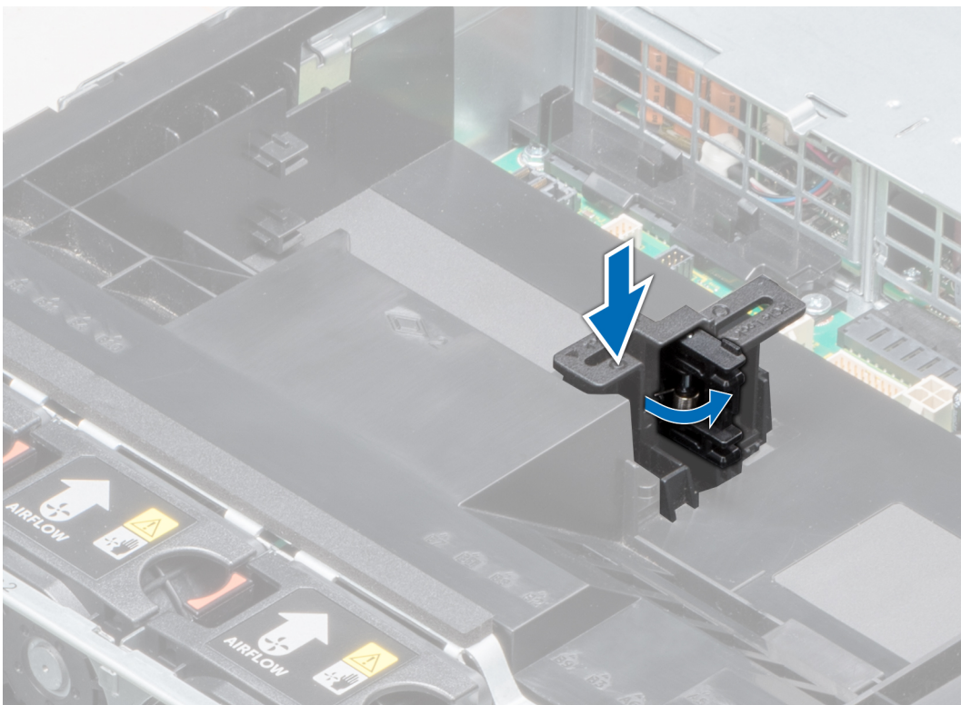
Figure 55. Opening the PCIe card holder latch
