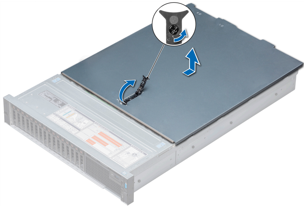
Figure 19. Removing the system cover
