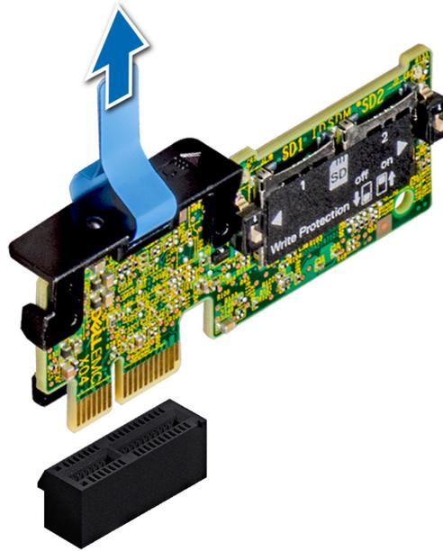
Figure 89. Removing the optional IDSDM/vFlash module
