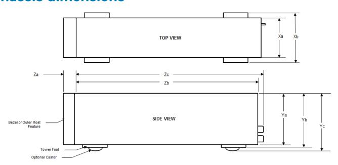
Figure 1. Dimensions of the Dell EMC PowerEdge T640 system
