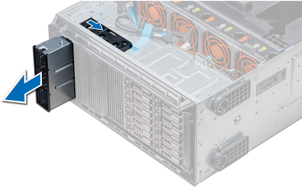
Figure 59. Removing the optical drive or tape drive
