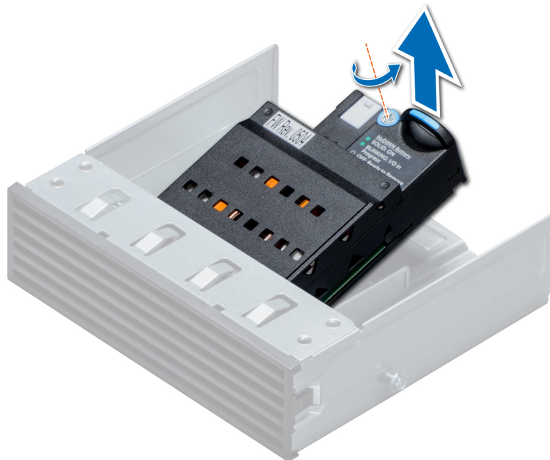
Figure 65. Removing the NVDIMM-N battery
