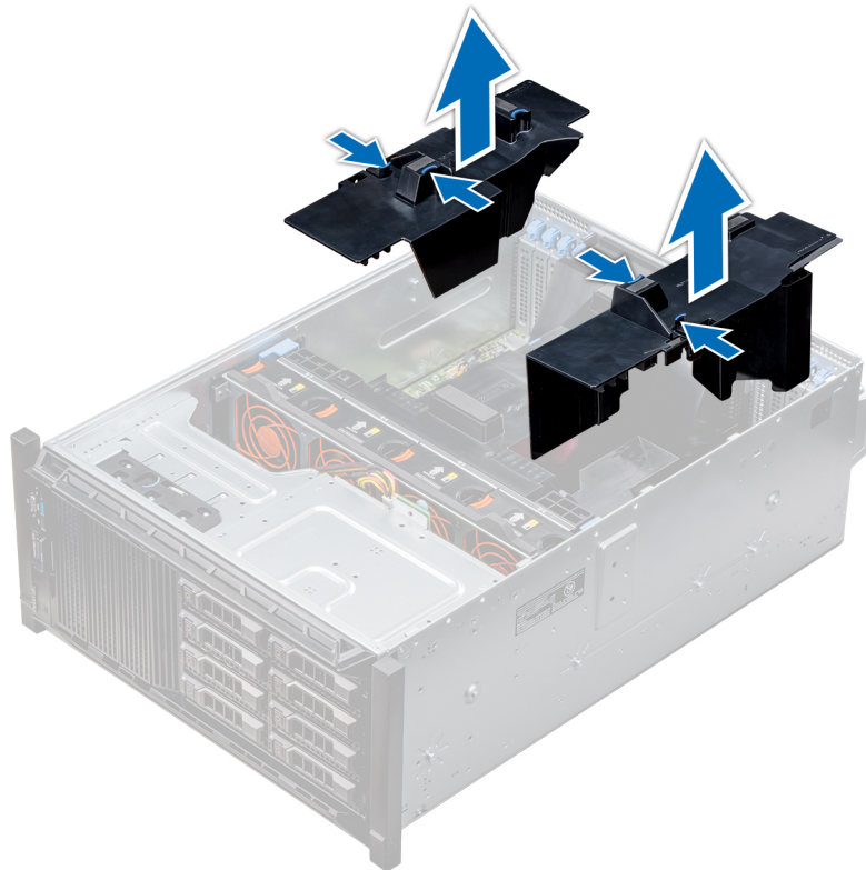
Figure 47. Removing the optional GPU air shrouds
