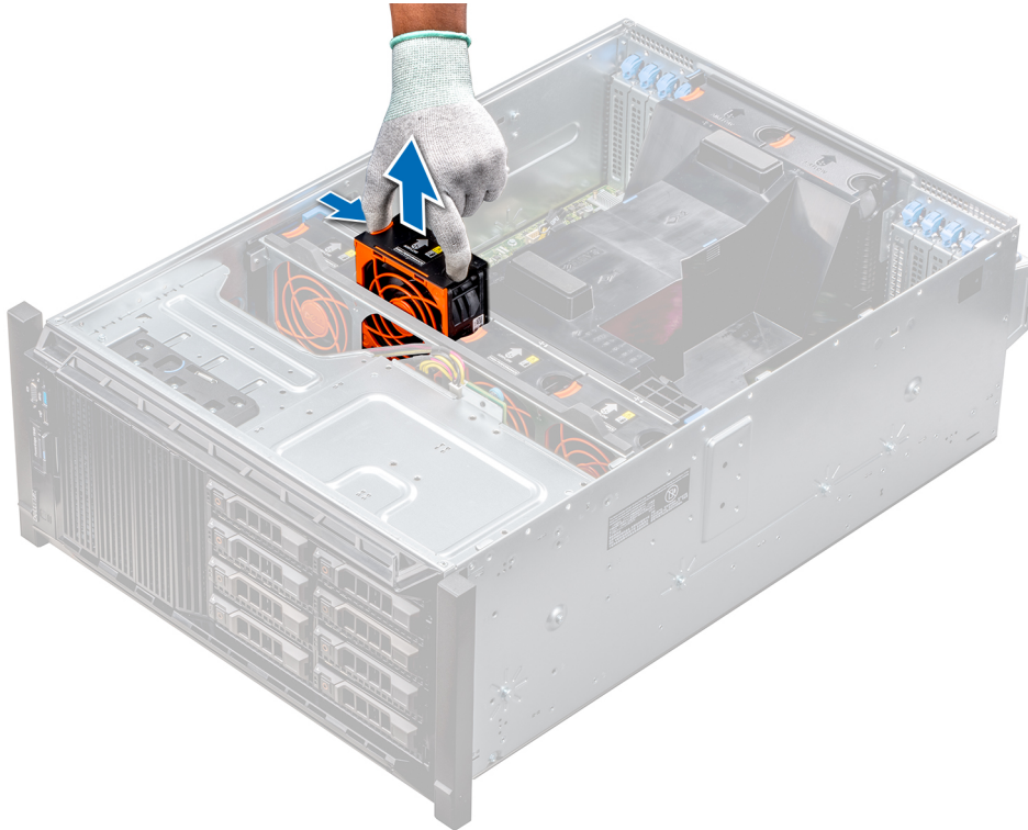
Figure 21. Removing a middle cooling fan
