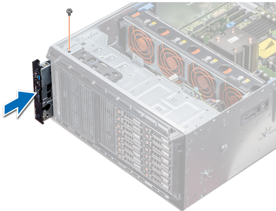
Figure 109. Installing the control panel assembly
