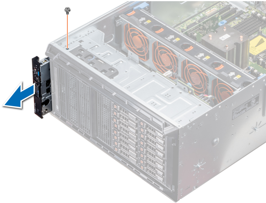
Figure 106. Removing the control panel assembly
