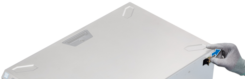
Figure 121. Attaching the mylar cover
