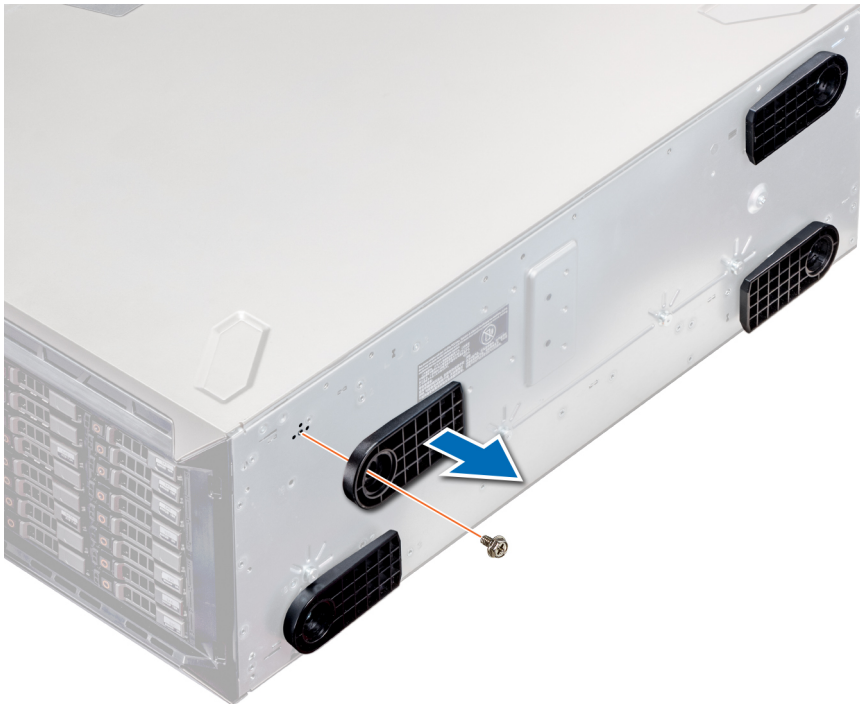
Figure 27. Removing the system feet
