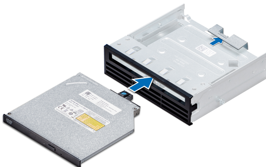
Figure 64. Installing the slim optical drive blank
