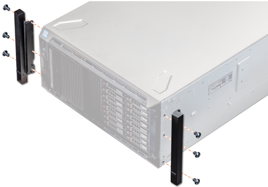
Figure 122. Installing the system ears
