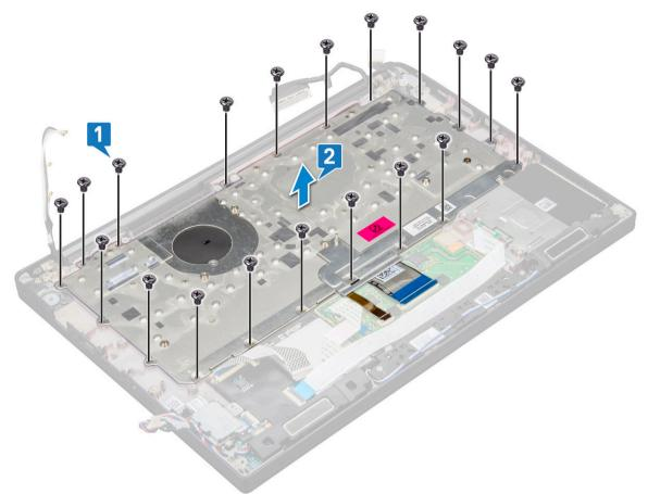
5 Remove the screws (5) that secures the keypad to the keyboard chassis and lift the keyboard [1,2].
