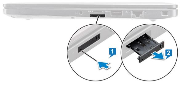
(i) NOTE: For Latitude 7390, the SD memory card must be removed before replacing any system components. Failure to remove the SD memory card before the disassembly of other components may result in damage to the system
