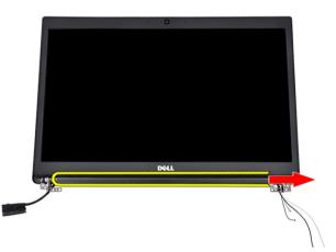
4 Remove the display hinge cap.
