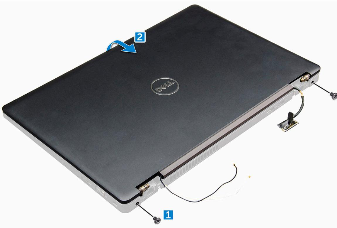
7 Lift the display assembly away from the computer.
