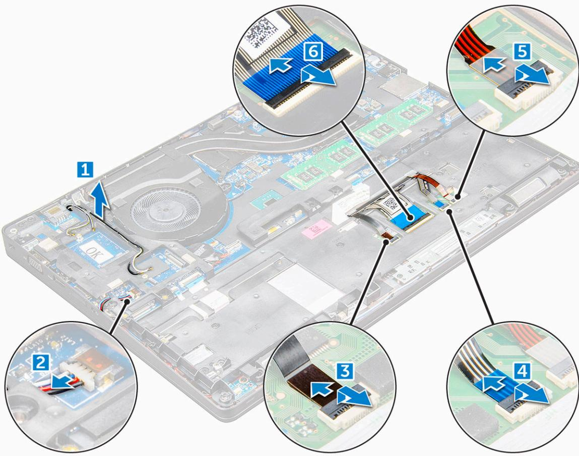
4 To remove the chassis frame:
