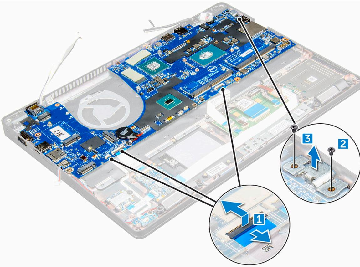
5 Remove the M2.0x3.0 screws and lift the system board away from the computer [1, 2].
